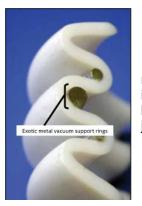
Internal vacuum support rings are available for larger expansion joints where they have a low or no vacuum performance. They will enable the bellows to work under full vacuum. These rings fit inside the bellows convolutions, so are exposed to the process. They are available either PTFE lined on the outside, or in various exotic metals. They may reduce movements of expansion joints, so please consult with us.
