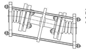
A tandem assembly of two expansion joints with an intermediate PTFE lined pipe provides wide lateral movements by effectively converting each expansion joint into angular types. Axial and angular movements are maintained further on.
